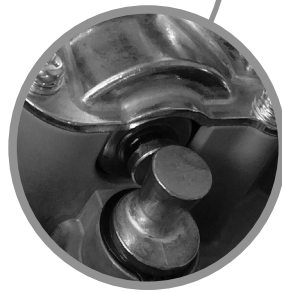
Position of unlocked motor : the pintle should be pressed
