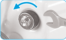
Loosen the 4 transport bolts with a spanner.
